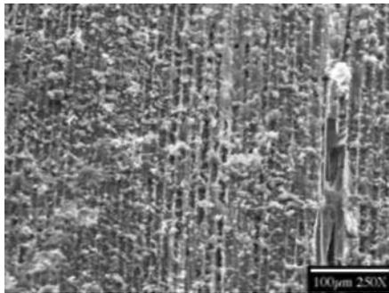
**Fig 7.** Laser-cleaned stem ( $0.56 \text{ J/cm}^2$ )
