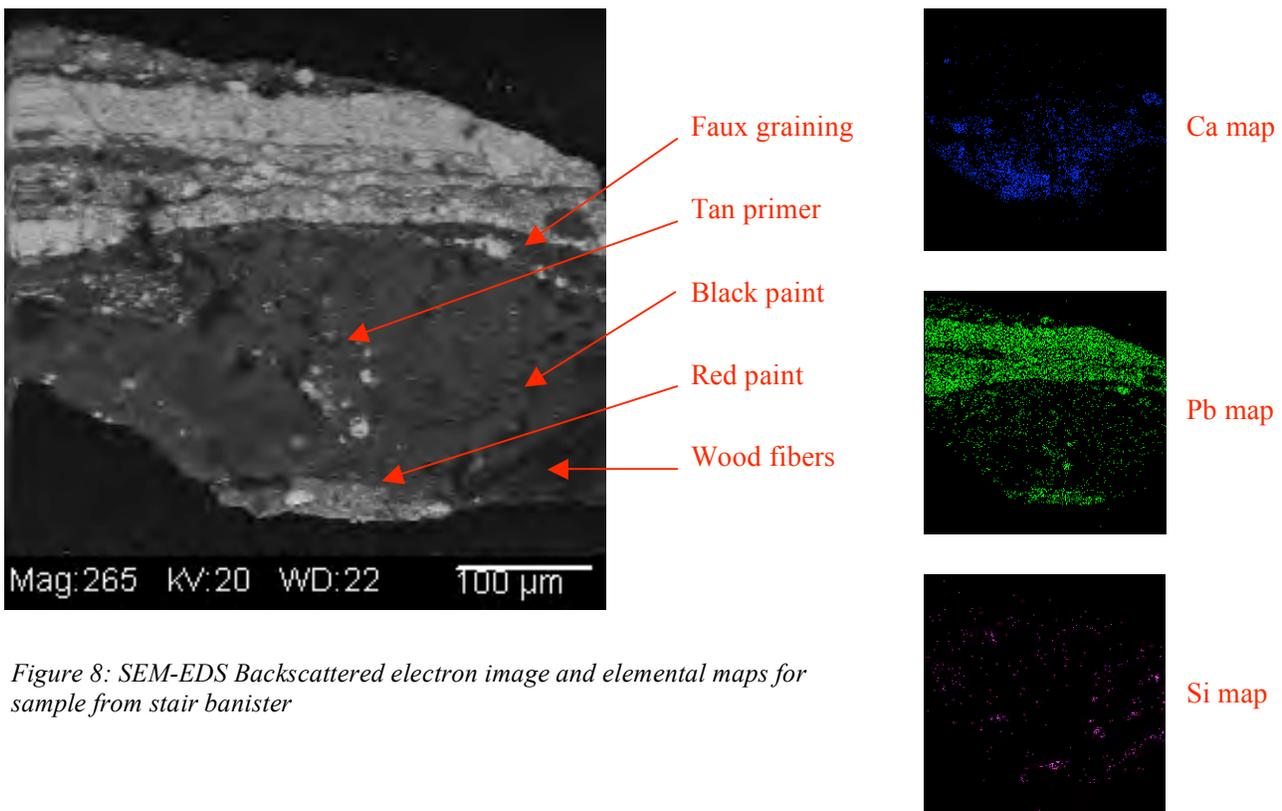
Figure 8: SEM-EDS Backscattered electron image and elemental maps for sample from stair banister
