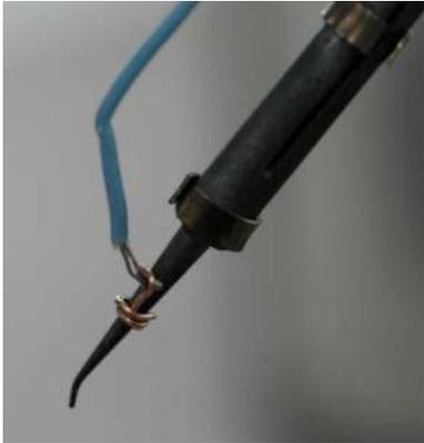
*Figure 8. A thermocouple attached to the hot needle with a copper wire*
