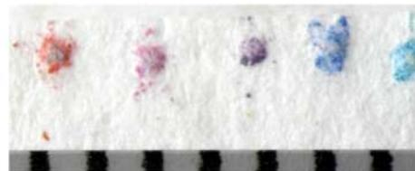
*Figure 10. Examples of the way crayons transfer to the photographic storage paper when tested with the hot needle (ruler indicates millimeters)*
