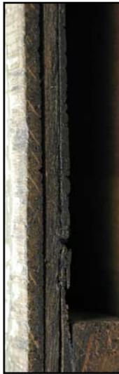
Visible rays on the end grain of the panel
