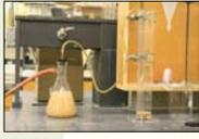
Removing clay from sand and silt
