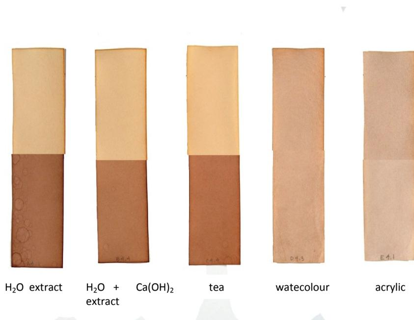
Figure 7 before aging images are above, after thermal aging images are below
