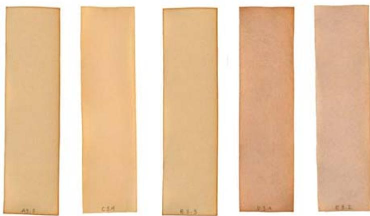
Figure 4 Prepared samples from left to right are: paper extract prepared with distilled water, extract prepared with alkaline water, tea, watercolour, and acrylic
