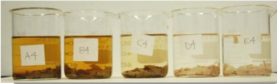
Figure 13 Samples soaking in distilled water after accelerated aging.
