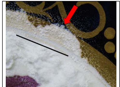
Figure 10. Detail photograph of the powdery residue that extended past the edge of the bleach application which is indicated with the black line.
