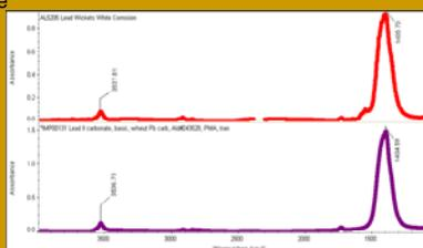
Fourier-transform Infrared Spectroscopy analysis: corrosion product from lead wickets (above) and reference spectra for basic lead carbonate (below)
