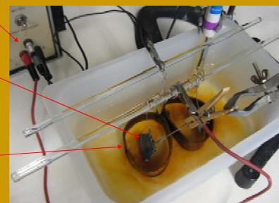
• Connection wires link anode and cathode to the power supply. Stainless steel wire links the anode and cathode to the connection wires.
