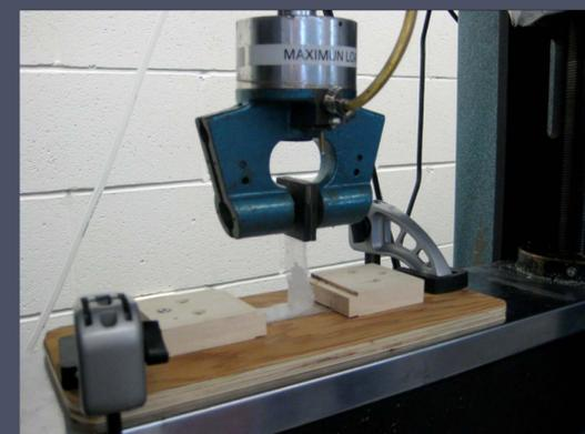
Fig. 5 Peel Test, Instron Tensile Tester
