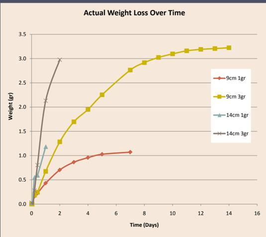
Fig. 3 Graph of sublimation rate of CDD aerosol spray. Actual weight loss over time
