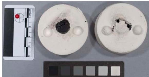
Plaster mold with bonded magnetic coating
