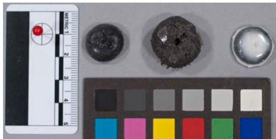
Elite Double 8 silicone rubber mixed with strontium ferrite powder (left) and iron filings (middle). Silicones Inc. P-4 silicone rubber mixed with equal parts strontium ferrite powder and chalk white (right).
