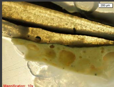
Fig 4. Cross-section of paint layers and foam under reflected light microscopy revealing layers consisting of paint, resin, paint, resin, paint, and foam.
