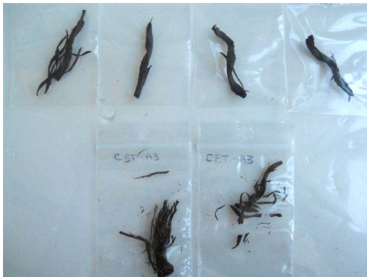
Figure 2. The top row of archaeological samples have been treated with sucrose. The bottom row were the untreated controls. One can see the difference in delamination and stability.
