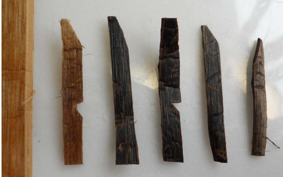
Figure 4. The colour change between the sample materials on the recto. From left to right, New cedar bark (never waterlogged), PEG-D4, ART-D2, ART-D4, ART-D6, CET-D4.
