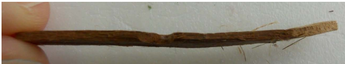
Figure 6. Illustrating the shedding common on the PEG controls
