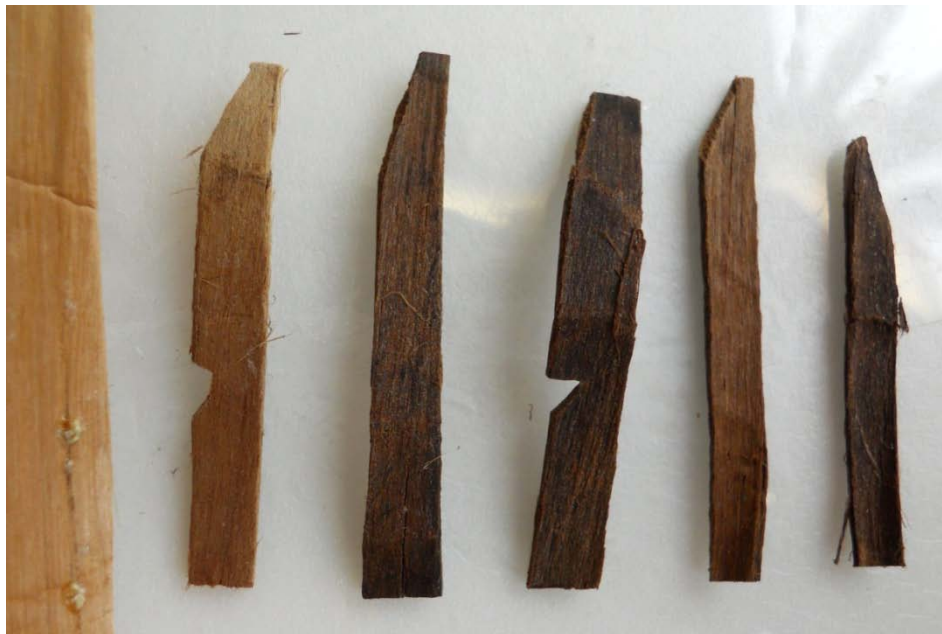
Figure 5. The colour change between all the samples on the verso. From left to right, New cedar bark (never waterlogged), PEG-D4, ART-D2, ART-D4, ART-D6, CET-D4.
