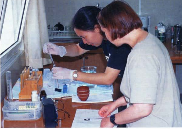
Figure 3: Measuring the conductivity of bath water during the desalination of excavated ceramics.
