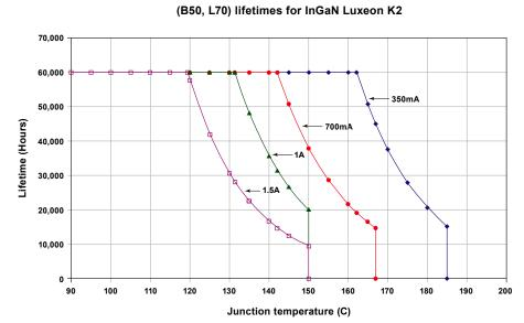
Figure 1. The curves show expected LED life based on drive current indicated by each colored line and target LED junction temperatures. Source: Philips Lumileds.
