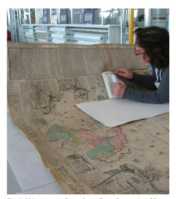
Fig. 10. Using steam on the overlap to allow safe separation of the text panels from the map
