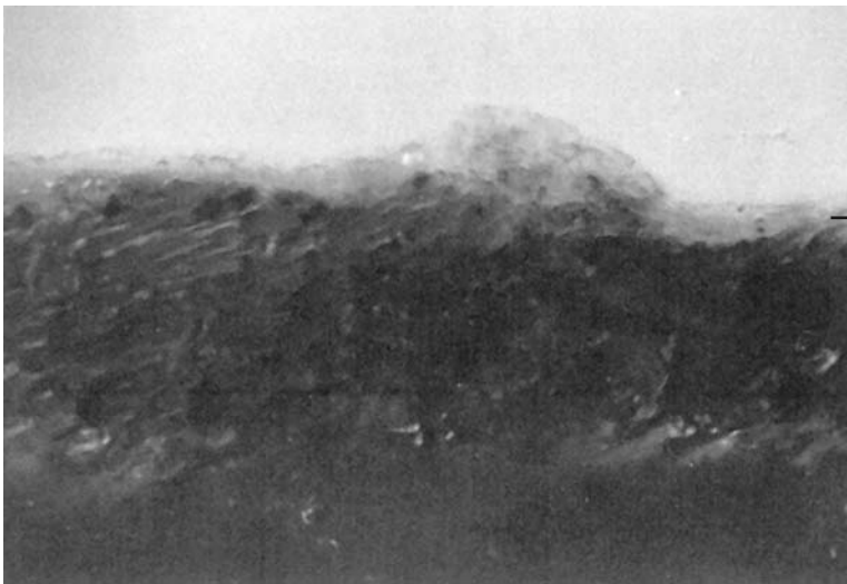
Figure 5. A synthetic varnish with flatteners was used on the wood surfaces in the studio and house to create a natural, matte appearance, but still provide a protective, washable surface. Top: UV light, bottom: visible light
