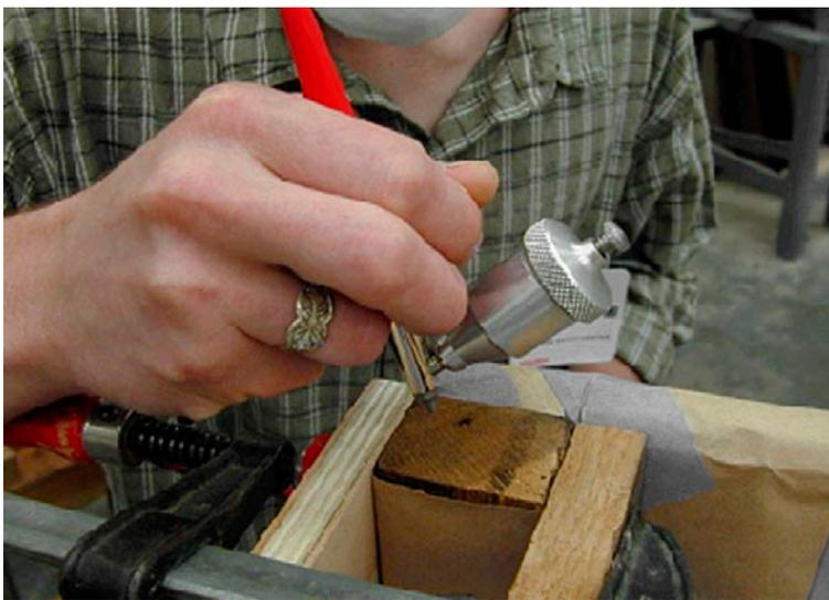
Figure 4. The apparatus for micro-abrasive blasting is similar to an airbrush, offering precise control and portability.
