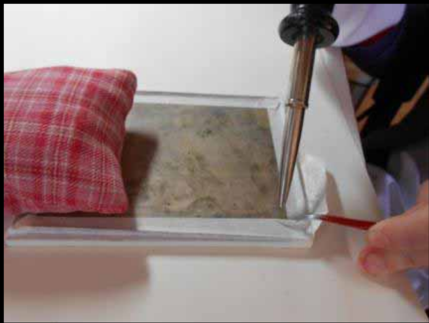
Removing non-original tape with hot air gun
