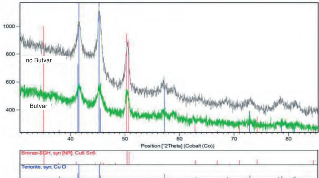
Similarly, XRD confirmed that tenorite was produced on both types of coupons, which suggests that the copper was oxidized in each case via the same corrosion mechanism (fig.5).
