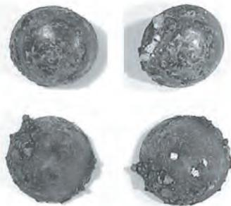
All of the studs developed bronze disease by the end of testing, which was confirmed by the presence of atacamite
