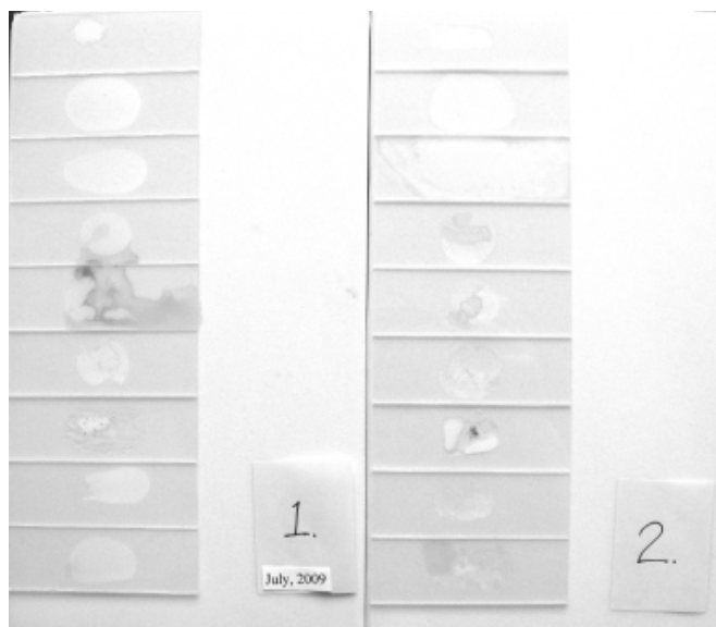
Figure 3. Experimental marble boards 1 (control) and 2 (cured at elevated relative humidity) four months after the application of UHU plus quickset epoxy. Faint pink discoloration formed on board 2, slide 3, the site of UHU plus quickset with excess hardener.
