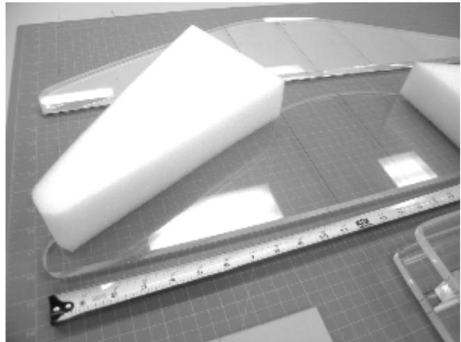
highly compact, archival filler. It also provides a porous surface to which layers of Ethafoam padding can be hot-glued, to cover the surfaces and edges of the acrylic sheet as well as the bolt heads.
